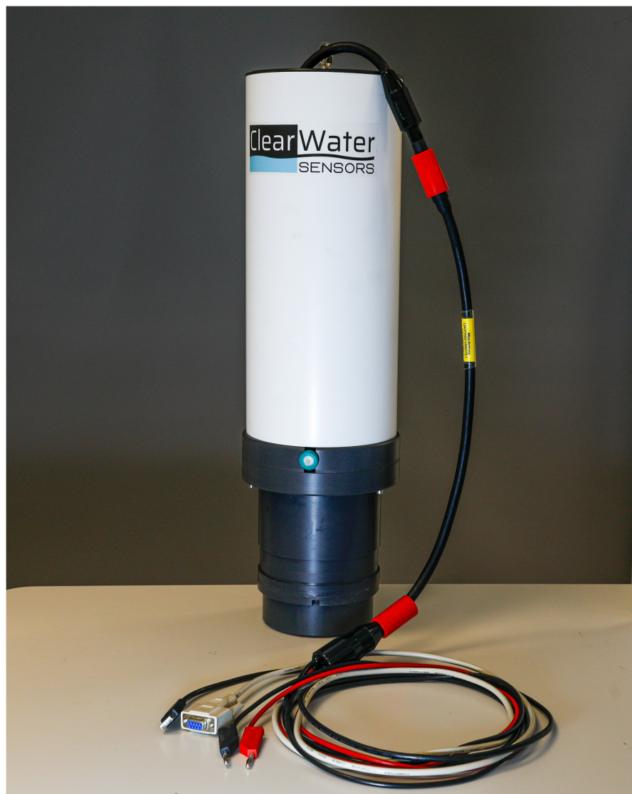
FIGURE 1 | Photograph of a silicate sensor (Clearwater Sensors Ltd., total height 56 cm) connected to a deployment cable which is then connected to a lab cable for connection to a bench power supply and PC for testing/calibration. The USB connection is used for setup and download of raw data, while RS232 can provide real time processed data in the field. The upper part including a larger gray collar and white tube is a reagent cartridge containing standards, blanks, reagents and waste storage capacity (all waste is captured). The lower gray cylindrical part houses the microfluidics, optics, pumps, valves and electronics (the sensor itself).
