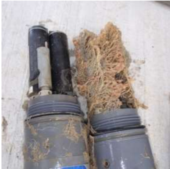
Figure 4. Distribution of biofouling on ProbeGuard equipped YSI (left) and control sonde (right) after retrieval from unattended sampling from 03/26/14 to 06/16/14.
