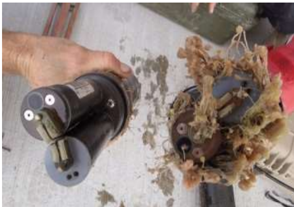
Figure 5. Optical sensor fouling on ProbeGuard equipped YSI (left) and control YSI (right) after retrieval from unattended sampling from 03/26/14 to 06/16/14.
