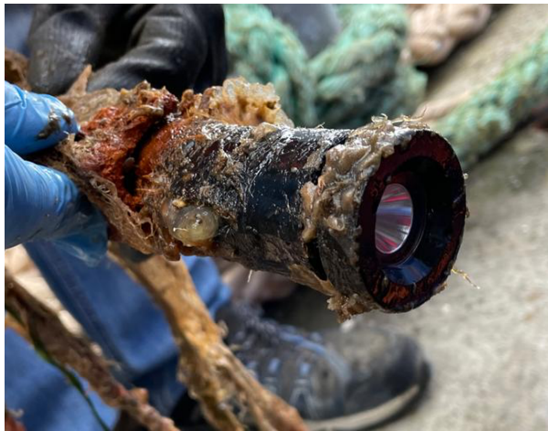
Figure 1. UV Lamp after 7 weeks under sea. The part of the lamp that irradiates UV light can be appreciated in a clean state.
